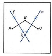
Construct the perpendicular bisectors  $\ell$  and m of  $\overline{AB}$  and  $\overline{BC}$ . Label the point of intersection D.
